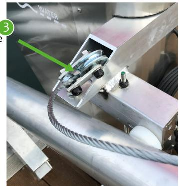
3 Thread the cable through the pulley
